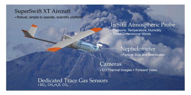
Figure 2: The SuperSwift<sup>™</sup>XT and its specialized payload.
